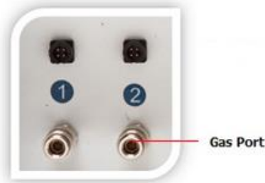
Figure 24.1 Gas sample ports
