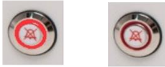
Figure 15.1 Alarm button that indicates the alarm condition
