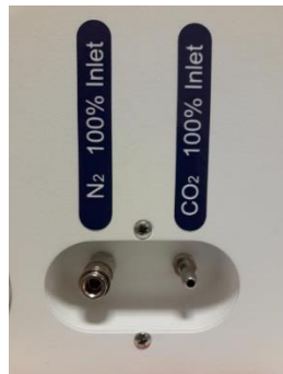
Figure 11.1 Gas inlets on the back of Mini MIRI® Dry and Mini MIRI® Humidity multiroom IVF incubators
