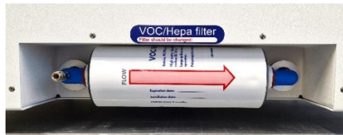
Figure 12.3 Correctly installed VOC/HEPA filter
