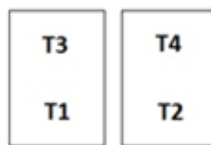
Figure 17.1 Temperature zones in the Mini MIRI® Dry and Mini MIRI® Humidity multiroom IVF incubators
