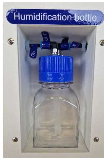
Figure 22.1 Tube connection on the humidification bottle and the Mini MIRI® Humidity multiroom IVF incubator
