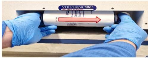
Figure 12.2 VOC/HEPA filter insertion and removal procedure
